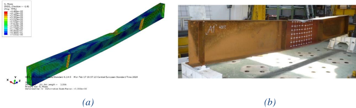
Fig. 18. Deformed shape of beam from both a) ABAQUS model and b) real test [46]
